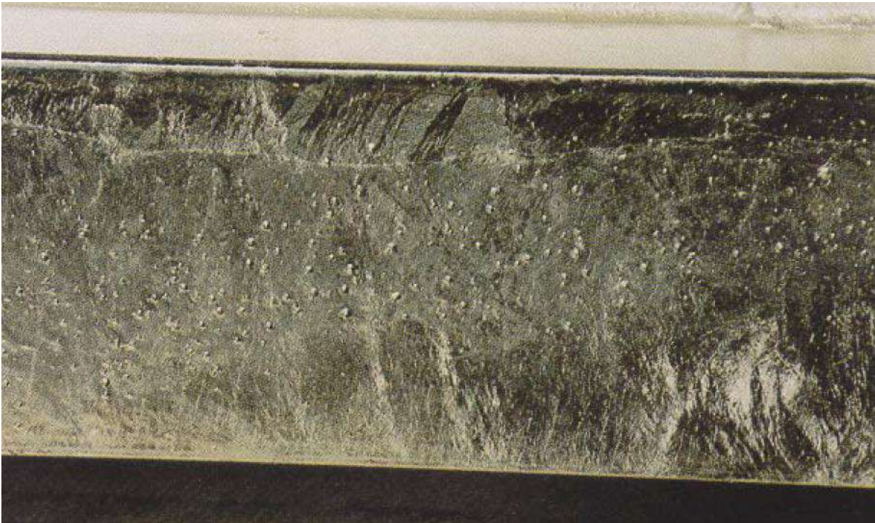
Imagen: Troubleshooting guideline. Dross pimples on finished products. American Galvanizers Association. Denver, Colorado, U.S.A., 2011.
